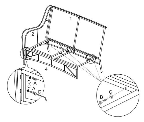
Use wrench (D) to secure love seat's seat frame (4) to love seat side frame (2) with bolt (A) and washer (C), and secure love seat's seat frame (4) to love seat back frame (1) with bolt (B) and washer (C).
