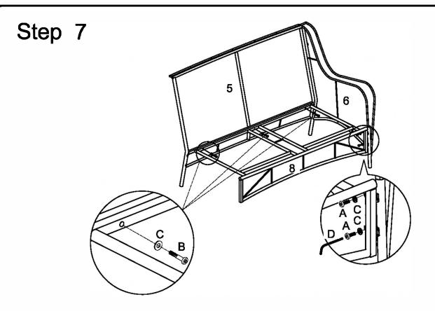
Use wrench (D) to secure love seat's seat frame (8) to love seat side frame (6) with bolt (A) and washer (C), and secure love seat's seat frame (8) to love seat back frame (5) with bolt (B) and washer (C).
