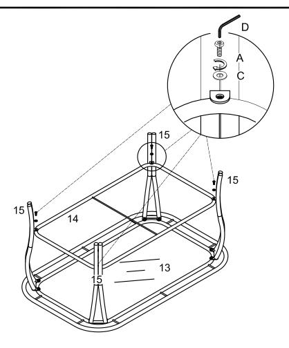
Use wrench (D) to secure shelf (14) to leg (15) with bolt (A) and washer (C).
