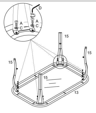
Use wrench (D) to secure leg (15) to table top (13) with bolt (A) and washer (C).
