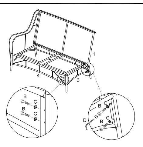
Use wrench (D) to secure love seat side frame (3) to love seat's seat frame (4) and love seat back frame (1) with bolt (B) and washer (C).
