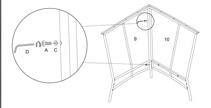
Use wrench (D) to secure corner seat back frame (9,10) together with bolt (A) and washer (C).
