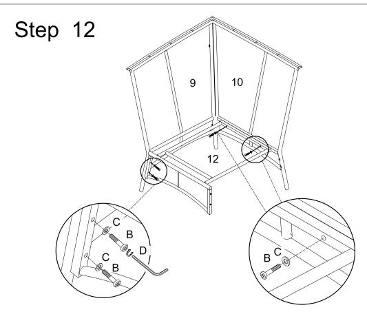
Use wrench (D) to secure corner seat's seat frame (12) to corner seat back frame (9,10) with bolt (B) and washer (C).
