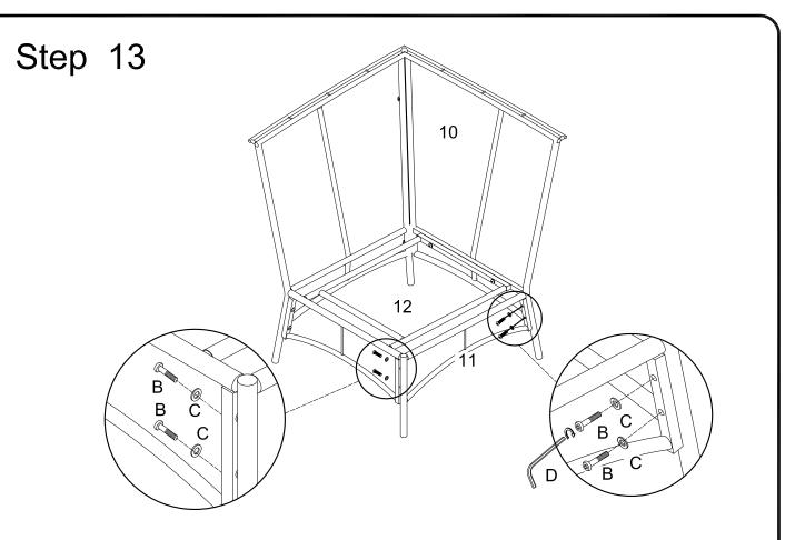
Use wrench (D) to secure corner seat side frame (11) to corner seat's seat frame (12) and corner seat back frame (10) with bolt (B) and washer (C).
