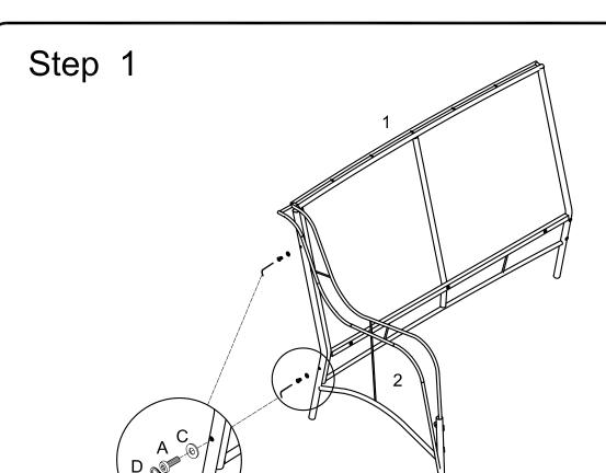
Use wrench (D) to secure love seat side frame (2) to love seat back frame (1) with bolt (A) and washer (C).
