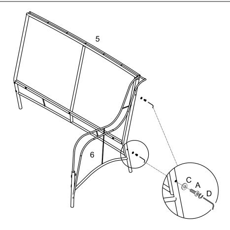
Use wrench (D) to secure love seat side frame (6) to love seat back frame (5) with bolt (A) and washer (C).
