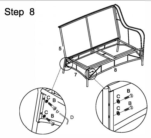
Use wrench (D) to secure love seat side frame (7) to love seat's seat frame (8) and love seat back frame (5) with bolt (B) and washer (C).
